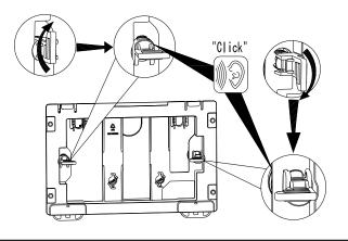
15. Please put the Adjustable Rod then push its back close to the wall.
