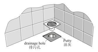
Please use scotch tape or other adhesives to seal the aperture around the floor drain after installation.
