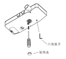
Remarks: If there is a small dimension (smaller than 10mm) difference between the faucet and the joint installation, please use a cross screwdriver to loosen (be sure not to unscrew) the screws slightly, then, screw down the screw after position adjustment.
