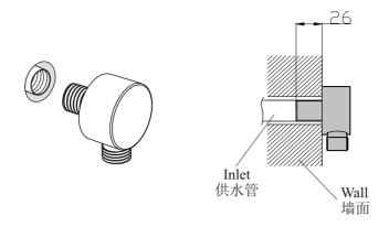
Connect shower hose to connect outlet and hand spray. Seal provide with hose must be installed in hose inlet end.
