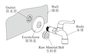
Install the bib tap into the Outlet on the wall.
