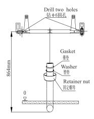
4.Move the tank from top to bottom while sticking closely to the wall, until it is placed into the tank bracket, and move the tank from left to right until the drain seat at the button snaps into the straight pipe. If the tank is slightly tilted, remove the tank and readjust the height of the side of tank bracket where the serrated gasket is located; then insert the retainer nut onto the thread of the tank button (discharge valve) and tighten.
