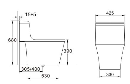
The size is for reference only, please check the actual size before installation 此尺寸仅供参考,安装前请仔细测量实际产品。
