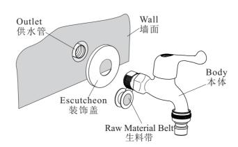
20190917 -1Install the bib tap into the Outlet on the wall.
