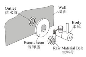
Install the angle valve into the Outlet on the wall.
