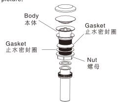
Insert the body of the rainspout from the water outlet of the basin, apply some sealant to the top of the drain of the basin and install the rainspout with water-tigh washer and fixing nut from the bottom of the basin. (Note: Don't do that with great impetus, to prevent breaking the basin.)
