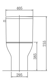
The size is for refernce only,please check the actual size before installation. 此尺寸仅供参考,安装前请仔细测量实际产品。
