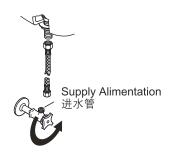
9 Flush several times and check for leaks.
